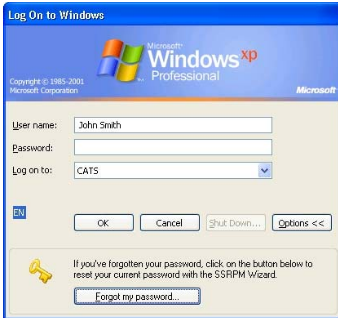
Figure 18: The 'Forgot My Password' shown at the bottom of the default Windows logon screen
